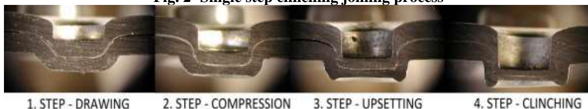
Fig. 3 Single step clinching process – the deformation of joined materials [1]
